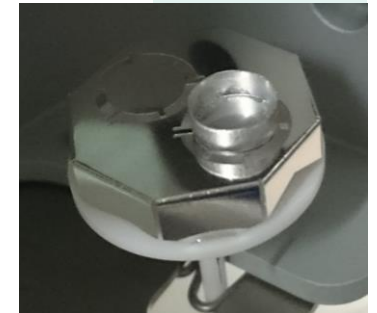
LFA liquid sample holder
