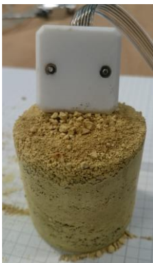
THB Sensor in compacted powder
