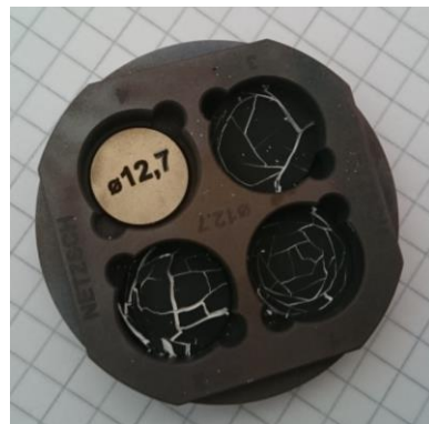
LFA samples with peeled of graphite coating
