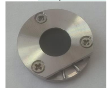
LFA liquid sample holder
