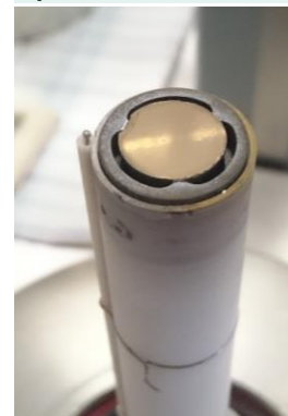
LFA sample with sputtered Au coating
