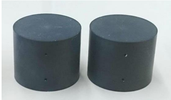
Referenzen aus Poly- etheretherkethon (PEEK)
